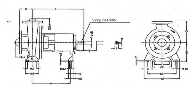
y: Distance between Motor Shaft and Pump Shaft
